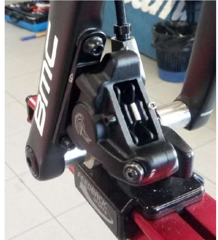
CAMPAGNOLO EC-DB013 bolts must be used to install the Campagnolo Super Record
